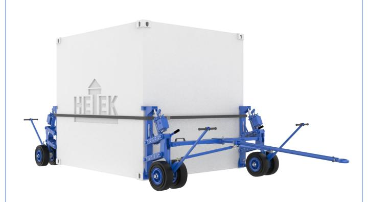
Lifting wheels series 507 up to 500mm stroke are suitable to move containers or modules up to 17t on little paved and lesser levelled ground. The assembling is to the frontside into the ISO corners, when the container is on standing the ground. To traverse the container has to be lifted up hydraulically by means of lifting wheels and can be moved from different vehicles. Using lifting wheels also small containers and structures can be loaded into cargo planes.
