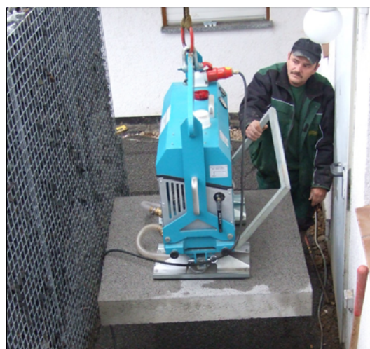
Kappa Levator with electric motor, carrying capacity 800 kg.
