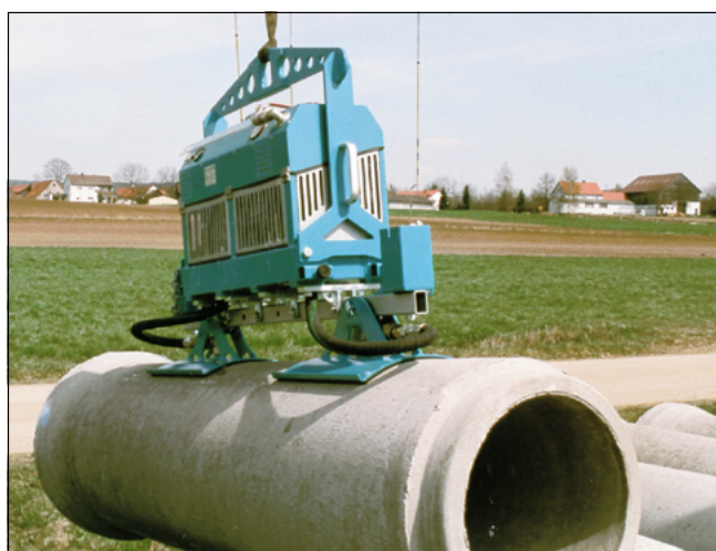
Kappa Levator with combustion engine, carrying module with 2 special suction pads for pipes of DN 500, carrying capacity 1,000 kg.
