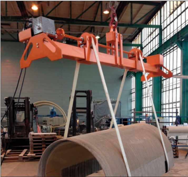
422 620 WTVE 2/2: Carrying capacity 2 t, working width min./max. 500/2,000 mm, adjustable with bolts, with counter weight
