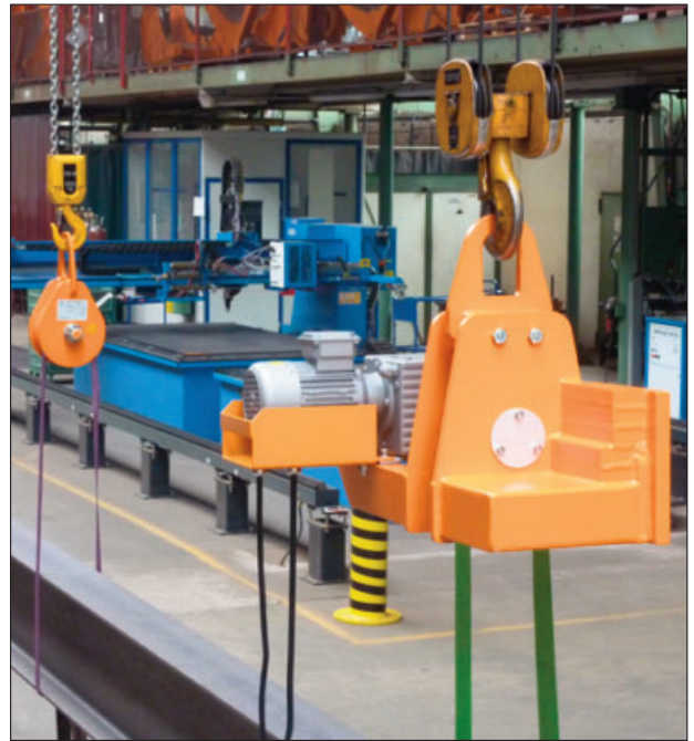
422 584 / 422 585: Load rotating device WTE 2.0 with load rotating drum WT 1.0, total carrying capacity 3 t
