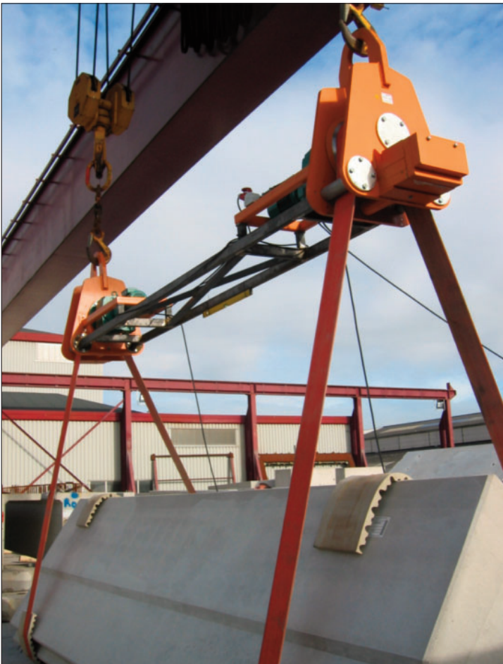
422 556: Two load rotating devices WG 12.5, with distance frame, total carrying capacity 25 t
