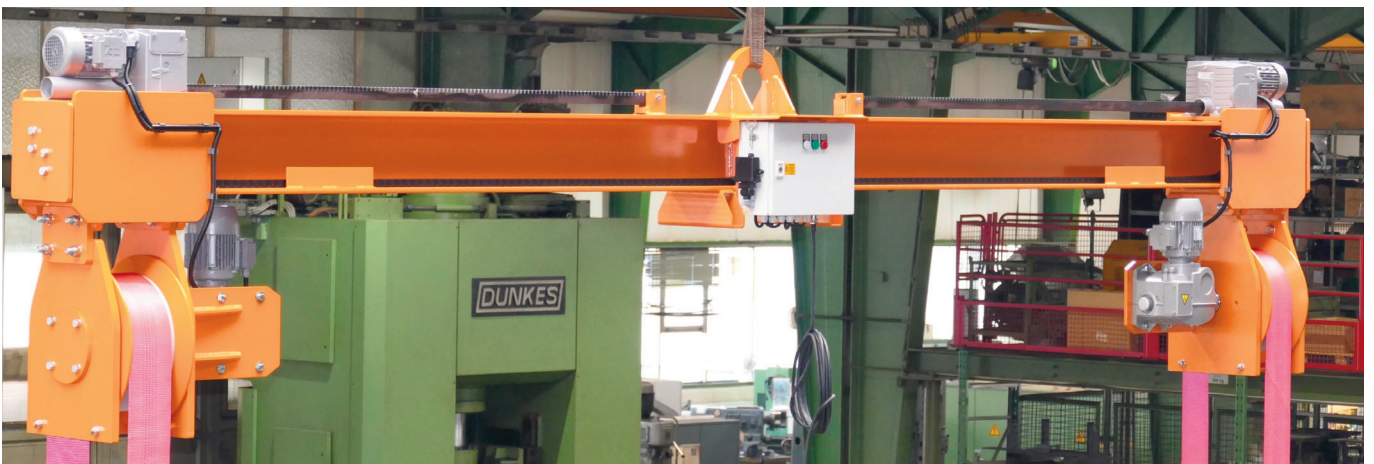
422 663 WTVE 10/5: Carrying capacity 10 t, working width min./max. 1,500/5,000 mm, electrically adjustable, with remote control
