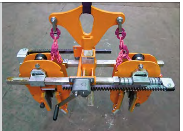
Pipe Grab RG 3,5 with simultaneous, stepless adjustment to the inside diameter via rack jack winch
