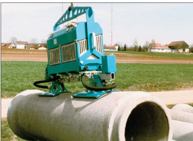
Kappa Levator with combustion engine, carrying module with 2 special suction pads for pipes of DN 500, carrying capacity 1,000 kg.
