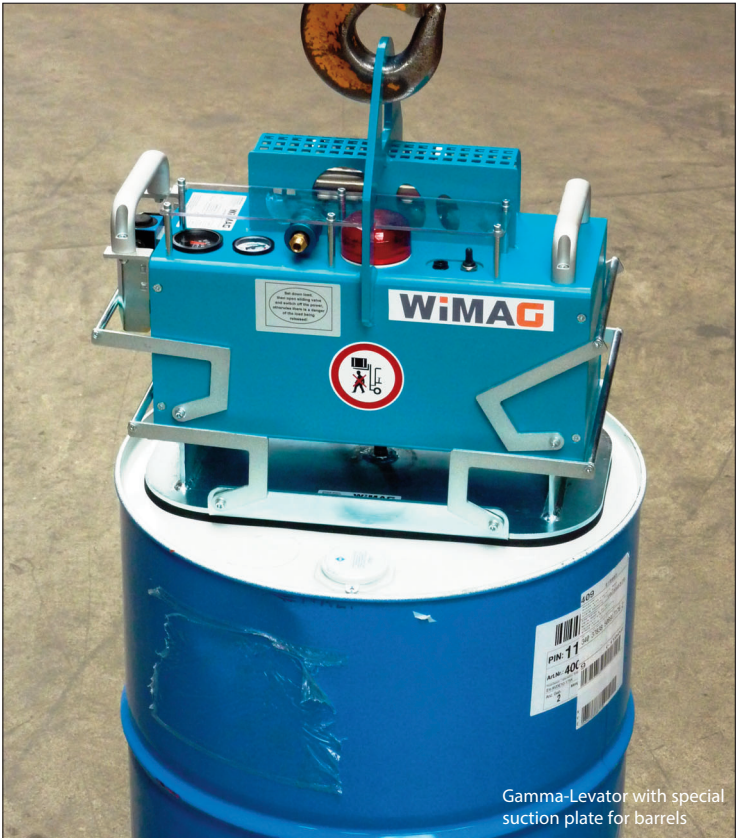
Gamma-Levator with carrying modul G2 and 2 suction plates
